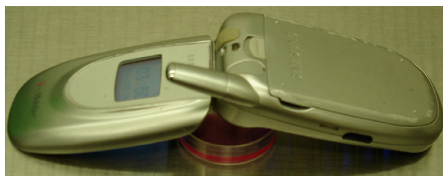
Fig. 1. Photograph of the method used to expose cultured cells to cell phone RF/MW radiation. The photograph shows a cell phone in “stand-by” or “on” mode placed on top of a 35 mm petri dish containing either primary neurons or astrocytes.
